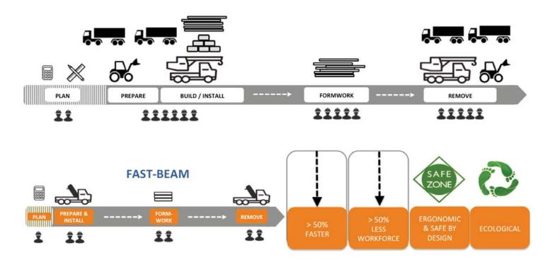
**Fast Beam** brings high-tech into bridge repair and maintenance operations. Fast Beam method replaces conventional scaffoldings used in bridge repair and maintenance operations. The adjustable Fast Beam scaffoldless method is suitable especially for edge beam preparation transforming any manual repair project into an industrial process. Expensive special skills are no longer needed.
